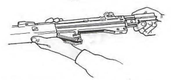
Check to be certain the operating handle is in the forward position. Then insert the complete bolt carrier assembly into the receiver as far as possible.
